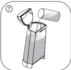
Fill the tank again with 0.65L of descaling liquid with MAX scale and repeat step 6 until the tank is empty.
