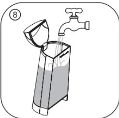
Empty and rinse the water tank. Fill with fresh potable water.
