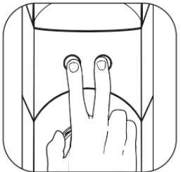
Press and hold both buttons for 5 sec in the same time to save and exit the volume setting.
