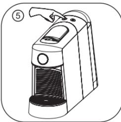
Press small button and plug on at the same time in power outages. Two lights flash (2time/ls).
