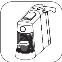
Press big button, 110ml coffee brewed. The big button blinks 1 time/s, small button keep long bright. (Press any button stop brewing coffee during this process)..
