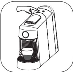
Press and hold the big cup (or small cup) button. Machine brew coffee until your desired volume is reached, then release button (finish volume setting).
