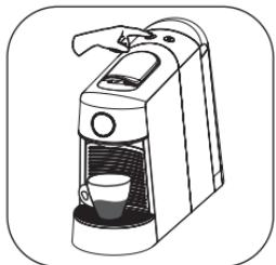
Press small button, 40ml coffee brewed. The small button blinks 1time/s, big button keep long bright. (Press any button stop brewing coffee during this process). Open the handle (capsule will drop into capsule box automatically).
