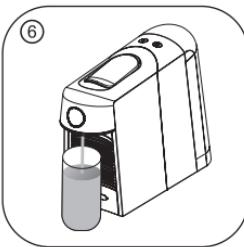
Press any key to start descaling until the water tank is empty.
