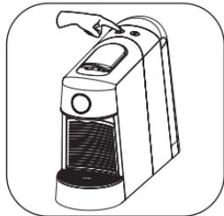
Press small button and plug on at the same time in power outages. Two lights flash (2time/ls). Enter descaling mode.
