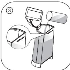
Mix the descaling liquid with the water as instructed. Fill the water tank up to the 0.65L line with potable water.
