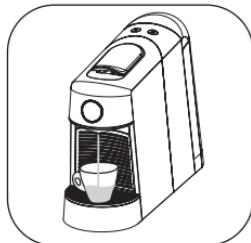
The indicator light of big and small button flashes at the same time, flashing frequency 1 time/second (the breath lamp is long bright).The preheating time is about 35s. Enter standby mode after preheating.First use or long time no use, please brew a cup of hot water to clean the machine.
