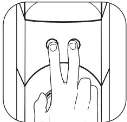
Press and hold big/small button 5s in standby mode, two lights flash ( 2 time /ls). Enter volume setting mode.
